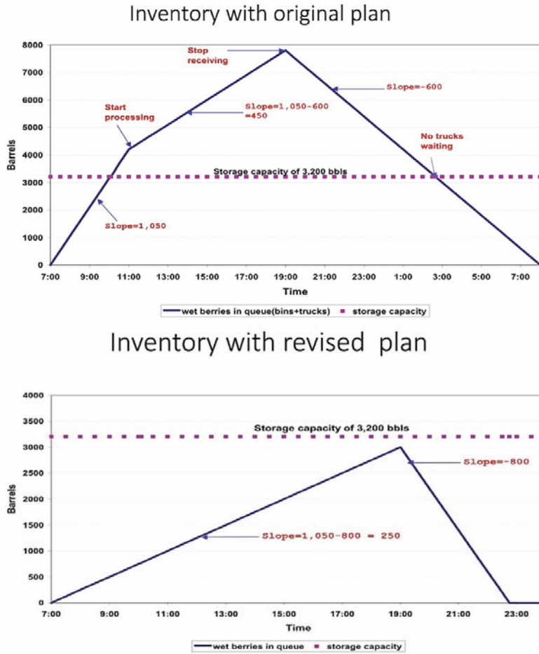
Figure 1. An example of the deterministic single-server fluid model applied to analyze the daily buildup and eventual decline of inventory over the day: a comparison of the original plan with processing at rate 600 bbl per hour starting at 11 (above) with a revised plan having processing at rate 800 bbl per hour starting at 7 (below).
